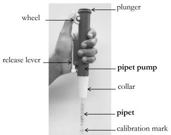
Figure 3. Pipet pump and pipet
